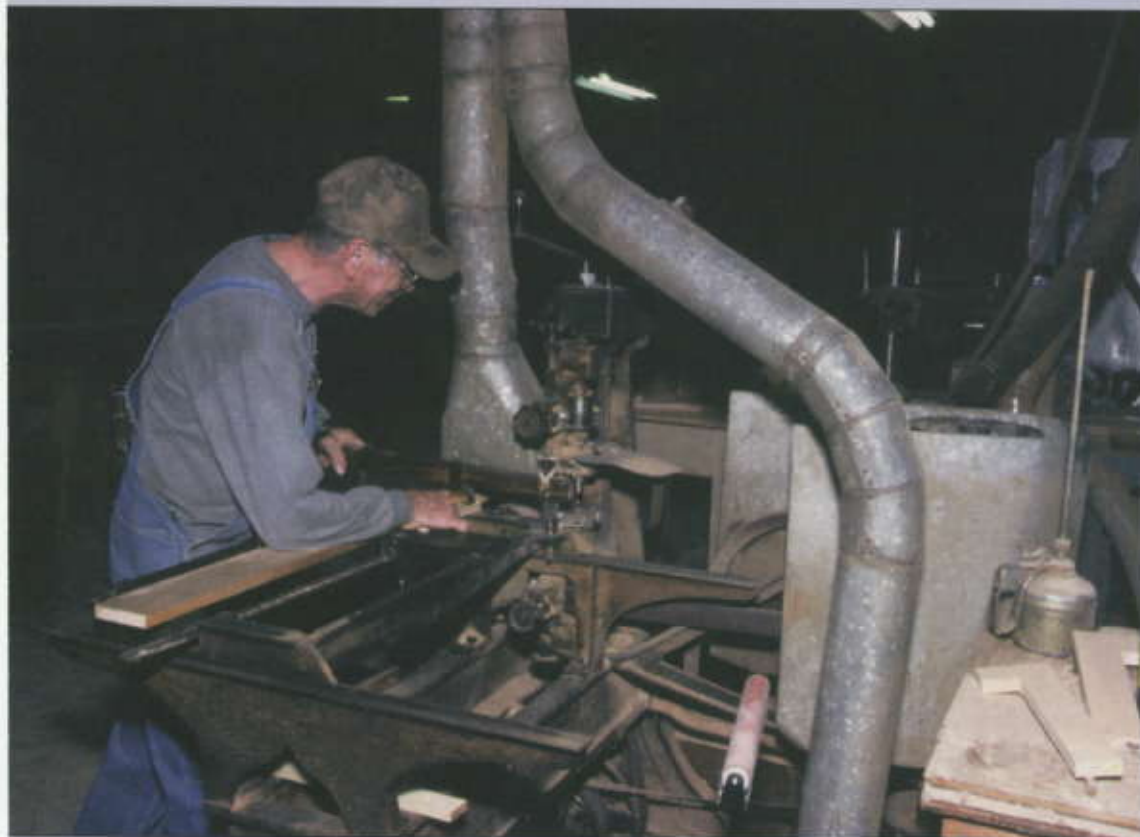
This hundred-year-old sash sticker machine was first powered by water and then converted to electricity in the 1930s. Coyle Lumber and Millwork continues to use this machine today to make custom window sashes.
